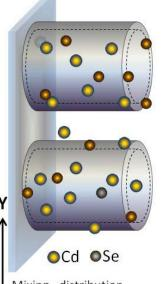
Mixing, distribution, and interaction between Cd and Se ions to form CdSe nanocrystals
