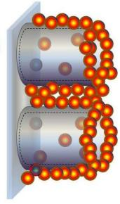
Orderly assembly and compaction of the preformed CdSe nanocrystals along T\_NT walls between 6-12 hrs.
