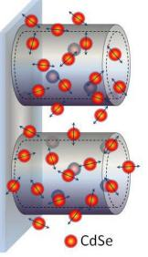
Formation of CdSe nancrystals and its random movement along XY axes in and around T\_NT over 6 hrs Growth of the preformed CdSe followed by its predominantly lateral movement along X axis
