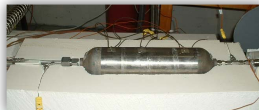
Cryogenic Adsorbent Component Test System
