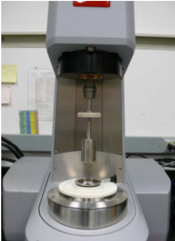
Anton Paar MCR301 rheometer with a bob/cup set-up
