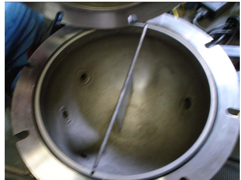
Figure 2: Two parts of the stainless steel sphere (8.8 liters free volume).
