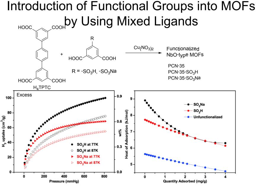
The SO<sub>3</sub>H group can be used as anchor for other metal incorporation
