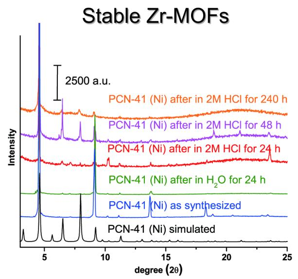
Strength of Zr-O coordination bonds prevents protonation of ligand under acidic conditions typically observed in MOFs.
