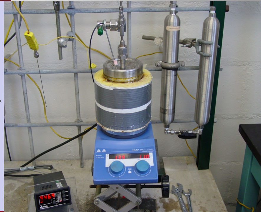
Oil bath - \text{H}_2 Desorption Experiment
