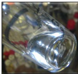
Picture @ Room Temperature Hexyl is Liquid = 0 C Hexyl is Solid = -40 C
