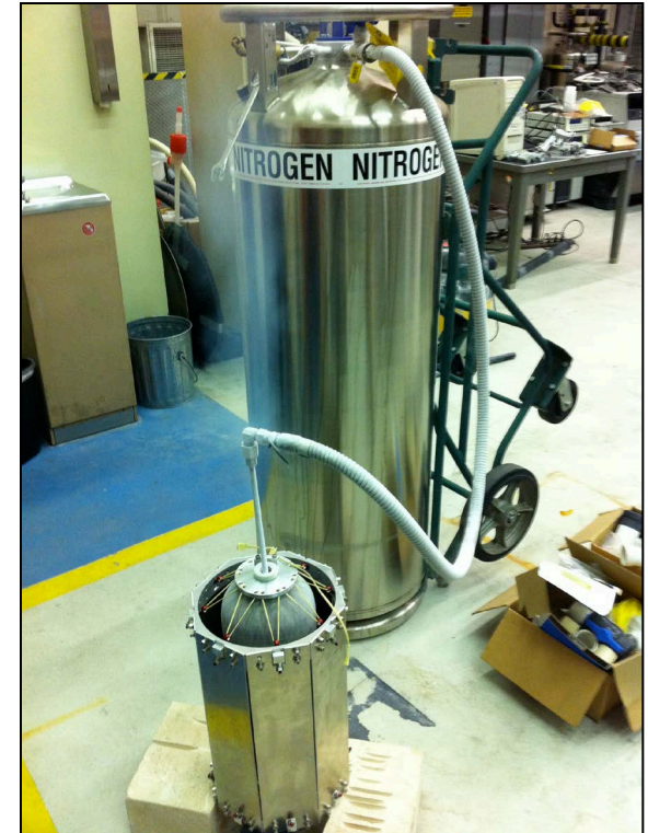
Image shows initial fill and testing of suspended tank article at LN 2 temperatures
