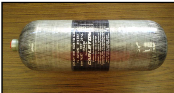
Glassfiber surrogate tank article and original CAD configuration model for test facility
