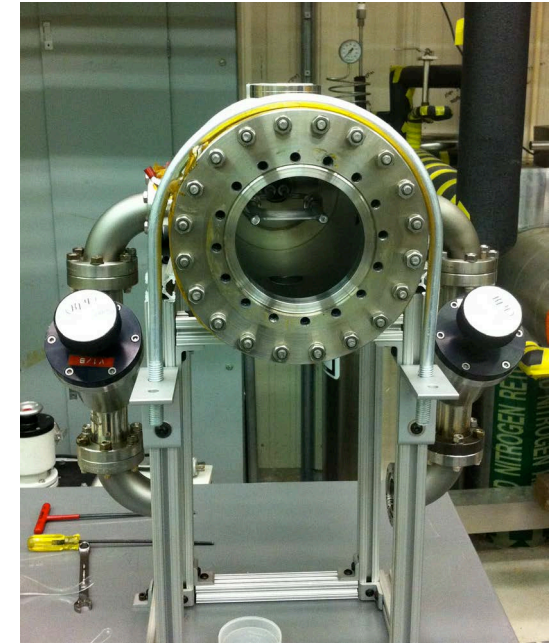
Outgassing facility under construction in JPL's H 2 Storage Engineering Laboratory. Sample stage can just be seen inside 8" chamber mouth. Facility has been assembled largely from existing hardware at minimal cost.
