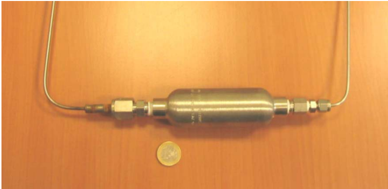
Small hydride test bed (150 g AB 5 ). Designed as a buffer tank for Room Temperature start up of PEM fuel cell.
