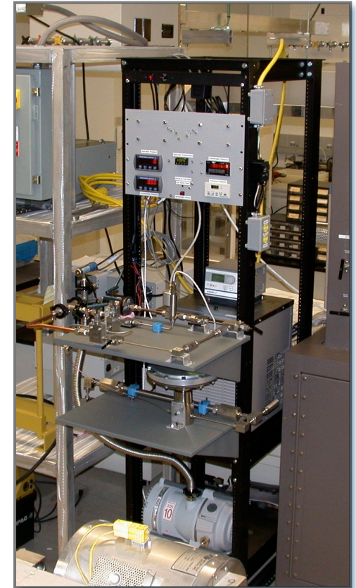
Improved temperature-cycling system – hydrogen manifold, high-pressure accumulator, temperature cycling controls, low-temperature chiller
