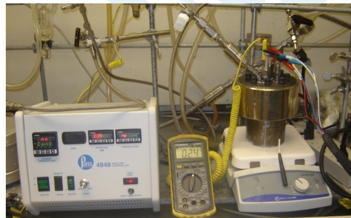
The Pressurized Electrochemical cell in operation
