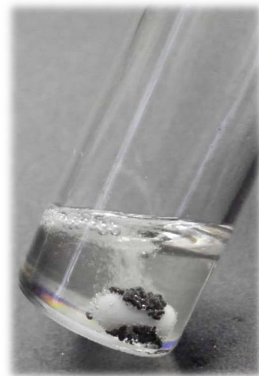
Catalyst particles (black) are on the surface of a magnetic stir bar.
