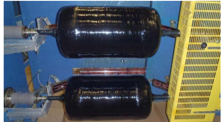
After the CNT reinforced epoxy resin was smoothed on the surface
