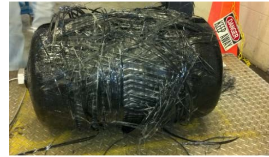
After burst test: Hydrogen storage tank reinforced with CNTs
