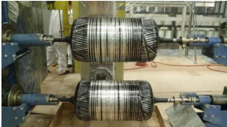
Glass fiber layer being wound with CNT reinforced epoxy
