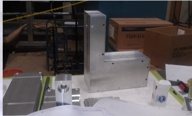
Figure 2: Side view of an assembled resin mixer during fit and print check.
