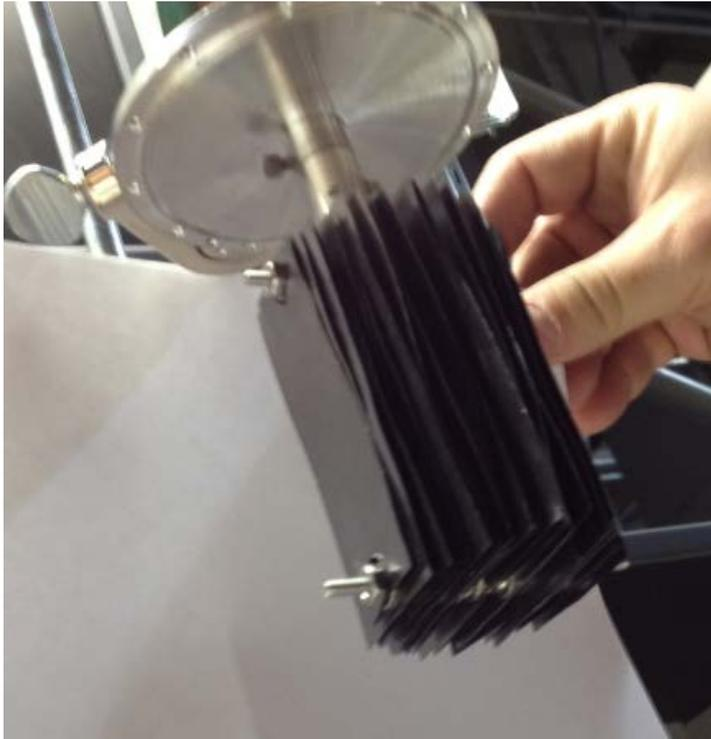
Sample for inelastic neutron scattering constructed of nominally parallel sheets of Grafoil® arranged with the cross section of an ellipse
