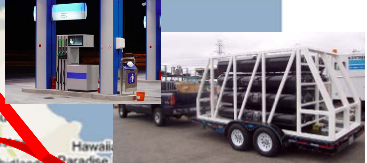
Hydrogen Delivery Trailer uses unique cascade fill process that required no onsite compressor
