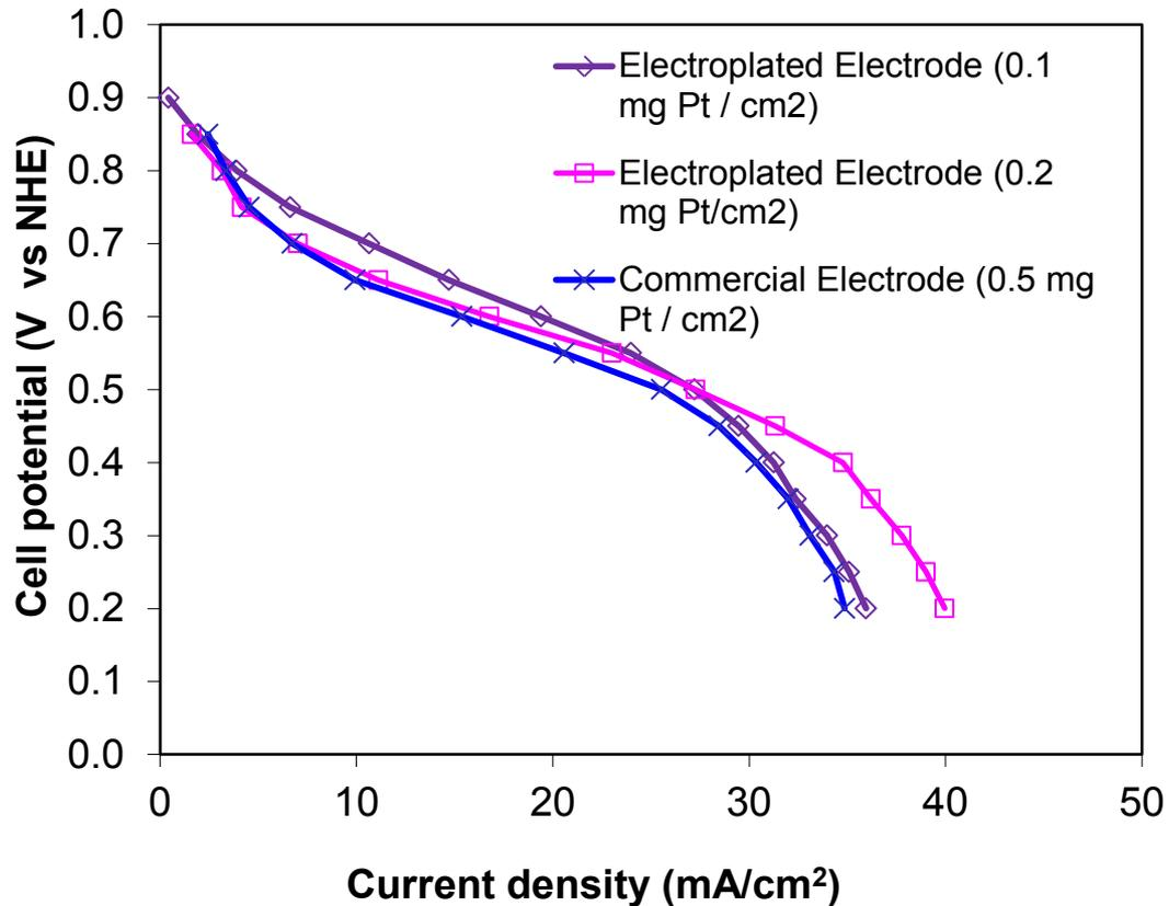
Comparison of ORR activity for electroplated electrode vs. commercial electrode
