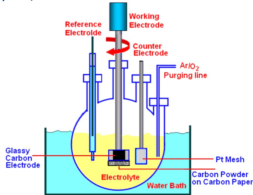
Figure 1 – Pulse electrodeposition and oxygen reduction reaction setup
