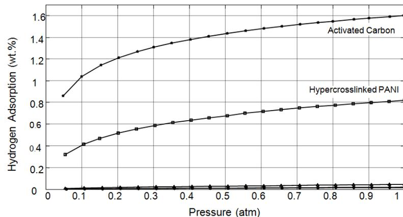
Hydrogen adsorption isotherms of PANI<sup>‡</sup>, PANI-G<sup>‡</sup>, PANI-GO<sup>‡</sup>, PANI-HYP and AC at 77.3K. <sup>‡</sup> Since PANI, PANI-G and PANI-GO performed almost identical they were not labeled but shown for comparison
