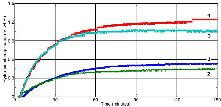
Absorption kinetics and storage capacity of different PANI samples at 70°C. (1 – 1M Aniline-1M CSA, 2 – 1M Aniline-0.5M CSA, 3 – 1M Aniline-0.05M CSA, 4 – 1M Aniline-0.01M CSA)
