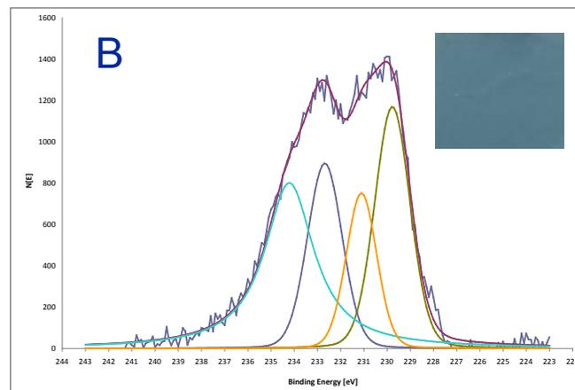
XPS spectra of Mo-based pigment before (A) and after (B) exposure to hydrogen
