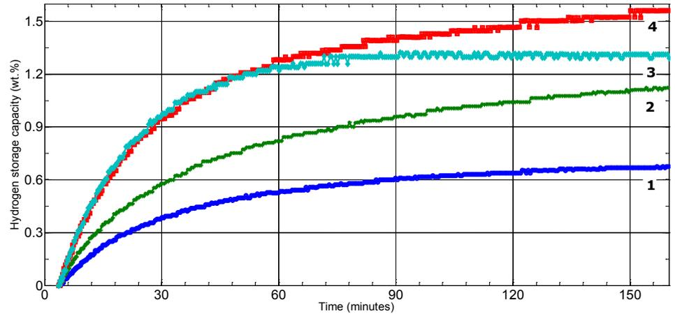
Absorption kinetics and storage capacity of different PANI samples at 25°C. (1 – 1M Aniline-1M CSA, 2 – 1M Aniline-0.5M CSA, 3 – 1M Aniline-0.05M CSA, 4 – 1M Aniline-0.01M CSA)
