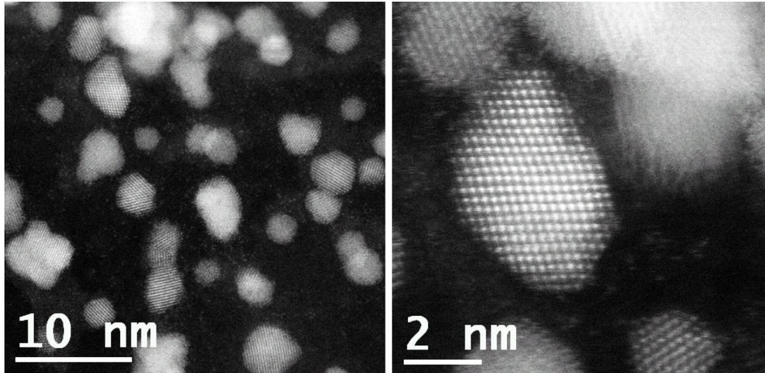
Figure 2 – Atomic level STEM of Nanosized Pt colloidal particles
