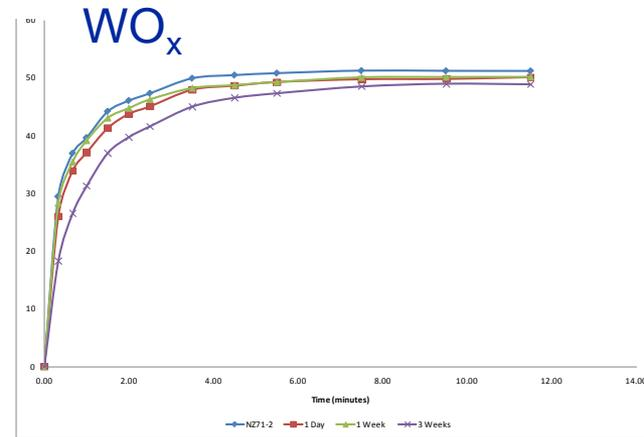
Effect of UV radiation (360 nm wavelength) on the performance of reversible Mo- and W-based hydrogen sensors. Exposure time: up to 7 weeks. Both sensors have good UV stability.  $\text{WO}_x$  shows faster response time.
