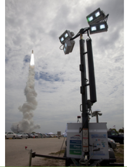
Hydrogen fuel cell powered light tower at Space Shuttle launch
