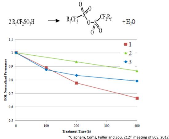
Water transport membranes (used for fuel cell membrane humidifiers) show decreasing water vapor transport properties with time. This has been assigned to anhydride formation in the membranes.
