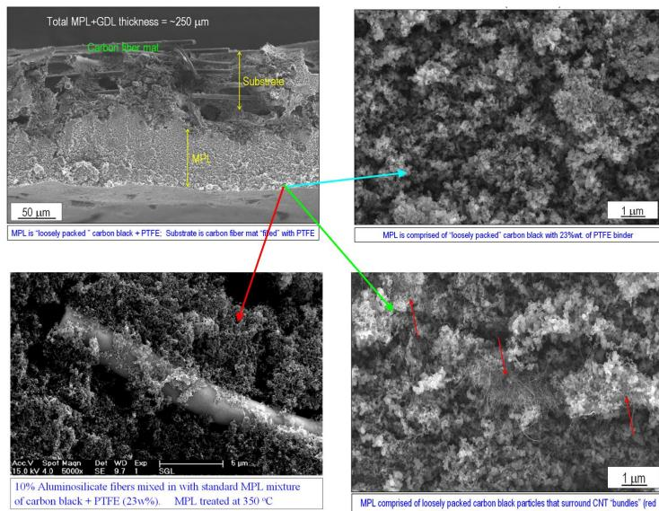
arrows) - CNTs are not homogeneously distributed within the MPL.
