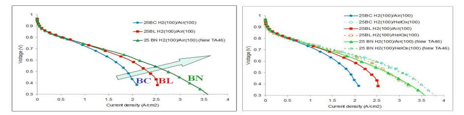
Performance improvement at high current for 25BL and 25BN in  $H_2$ / Air. Similar performance for 3 GDLs in  $H_2$ / HelOx (O<sub>2</sub> diffuses 3.7x faster in He vs. N<sub>2</sub>)
