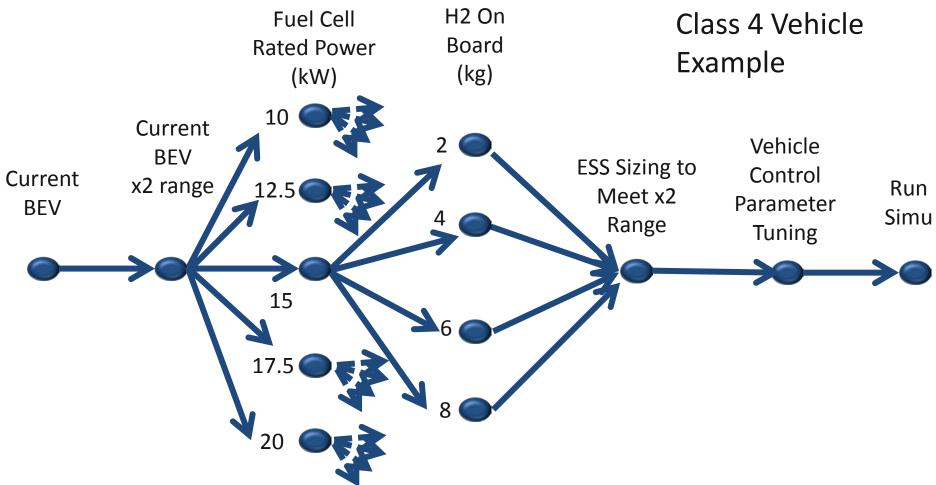
2 BEV + 5 Fuel Cell rated Power \* 4 H2 On Board = 22 Vehicles All vehicles sized to meet similar Vehicle Technical Specifications
