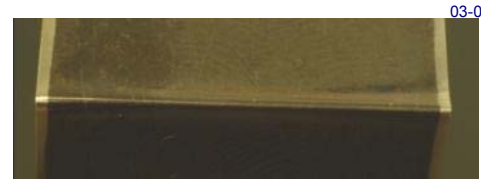
Example of good coating after bend test
