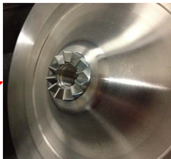
Curvic Spline Couples Rotor to Drive Shaft
