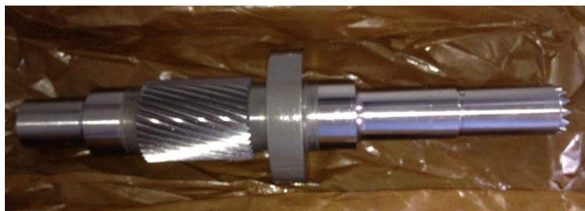
First Stage of 6-Stage Compressor and Drive Shaft with Pinion and Thrust collar
