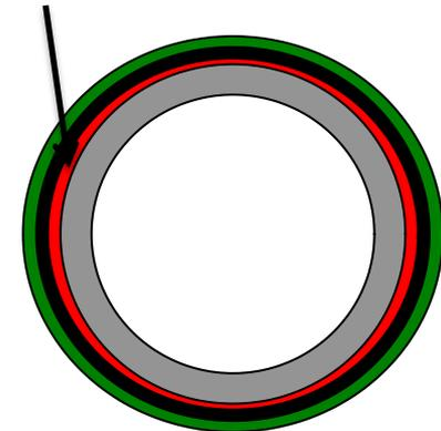
A small eccentricity may still exist after insertion of coupling resulting in uneven O-ring compression and partial extrusion
