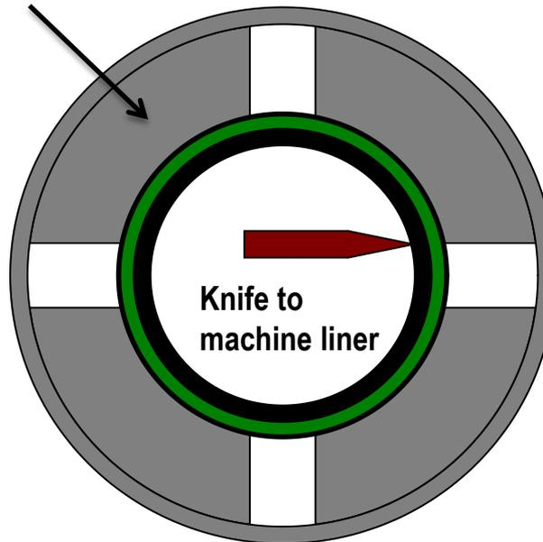
A 4 jaw chuck system is used bring FRP concentric where liner is machined to coupling diameter
