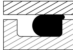
Illustration of O-Ring Extrusion
