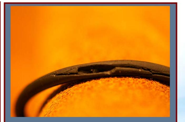
O-Ring Damage 3000 psig Fatigue Test
