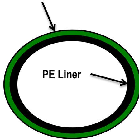
FRP Cross-Section Initially has a slight oval shape
