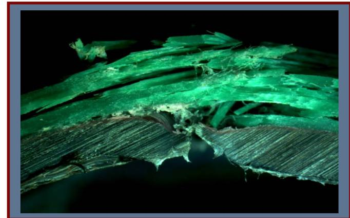
Cross-Section View Through Crack
