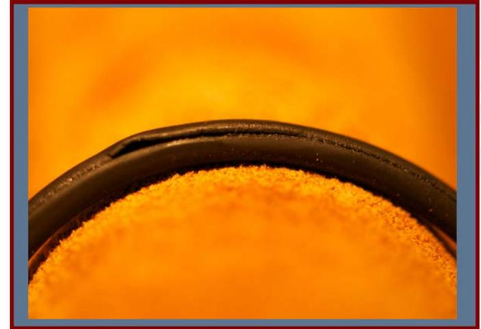
O-ring Damage 750 psig Fatigue Test
