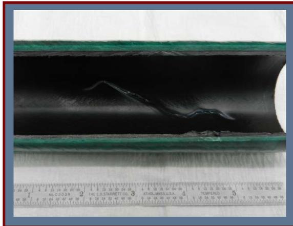
Inside View Showing Rupture of Liner
