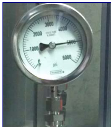
Hydrogen at 5,000 psig (Ambient O 2 ) Generated directly in PEM Electrolyzer
