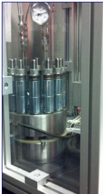
Hydrogen at 5,000 psig (Ambient O 2 ) Generated directly in PEM Electrolyzer
