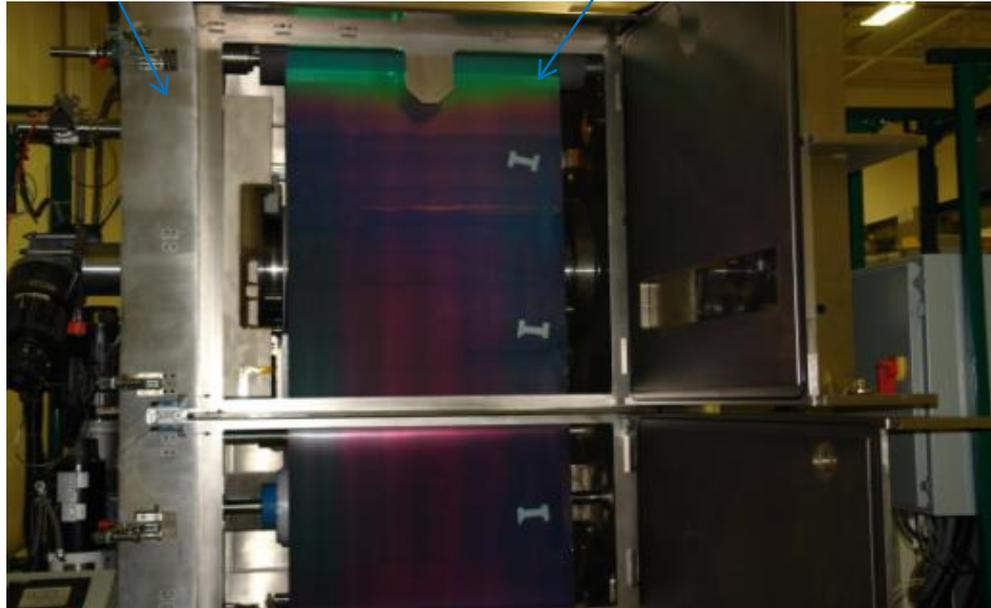
Opened pay-out chamber of the 2 MW-line with inserted stainless steel web after sputtering of  $\text{Co}_3\text{O}_4$ :
