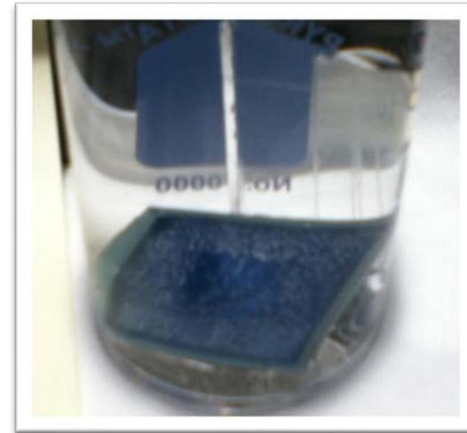
(b) PEC electrode with  $Co_3O_4$  on top of ITO
