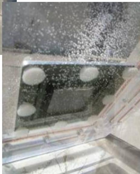
On the backside of the PEC electrode vigorous  $H_2$  evolution was observed;
