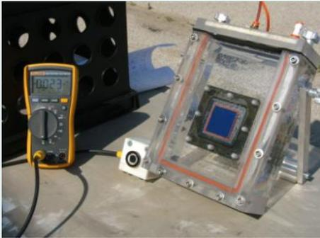
A photograph showing a square-shaped PEC cell mounted in a metal frame. A yellow multimeter is connected to the cell, and a power source is visible in the background. | Front and back side                   | 5.7%                    | TCCR<br>Materials | Main subject of this research         |
