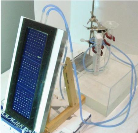
A photograph showing a rectangular PEC panel with a grid of small cells. It is connected to a power source and a multimeter, with blue tubes for electrolyte flow.    | Only back-side                        | 5.0%                    | Cost reduction    | Down-selected due to budget reduction |
