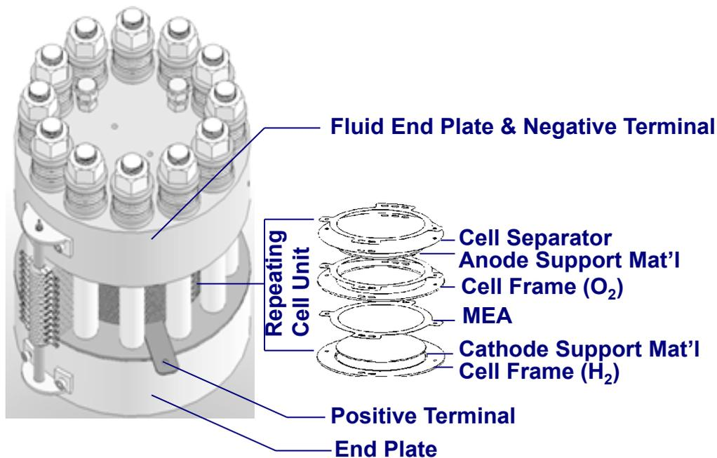
The repeating cell unit comprises >90% of electrolyzer stack cost
