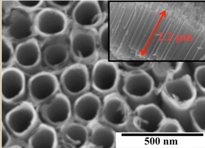
SEM TiO<sub>2</sub> NTs formed at 40 V for 1 h in an ethylene glycol solution (10 wt% H<sub>2</sub>O + 0.5 wt% NH<sub>4</sub>F) without any surface treatment prior to anodization
