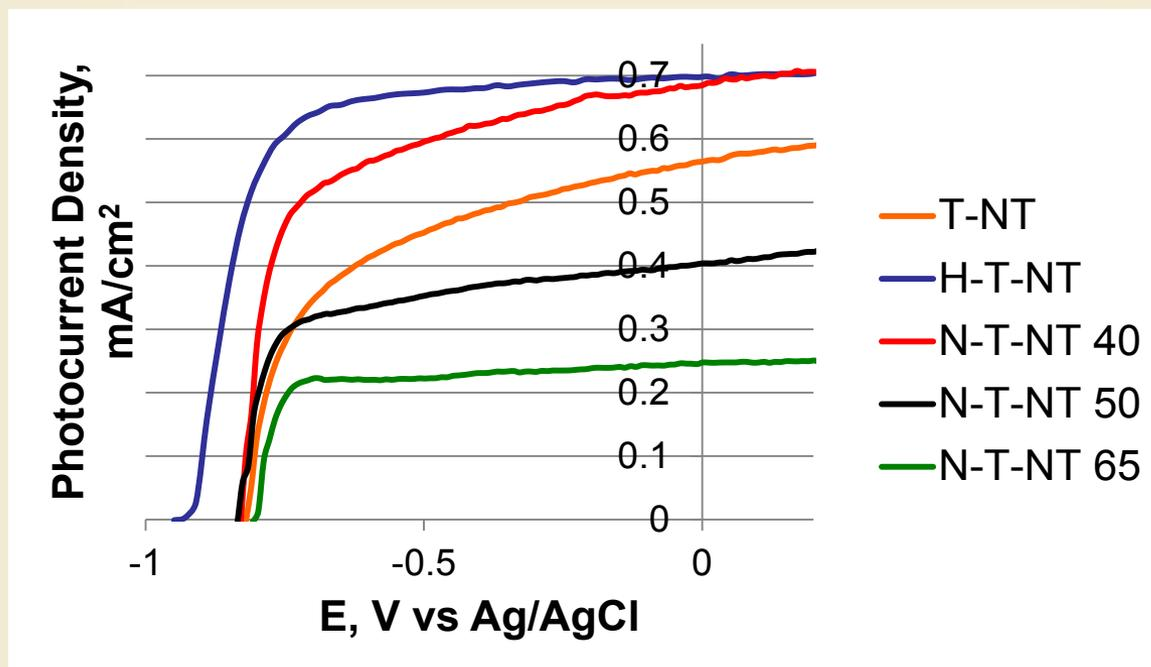
The increased performance of H-T-NT and N-T-NT 40 can be attributed to an increase in surface area for light harvesting and electrolyte interaction sites. The addition of a thin top layer can increase the workfunction over plain TiO<sub>2</sub> NT [3]. Too thick of a layer (eg N-T-NT 50) results in increases electron-hole recombination
