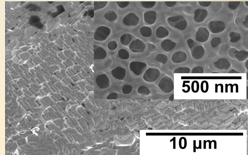
SEM of Ti surface after etching treatment. The inset shows the surface morphology after anodization at 40 V for 1h. The etching treatment results in the formation of a thin nano-porous layer on top of the TiO<sub>2</sub> nanotubes
