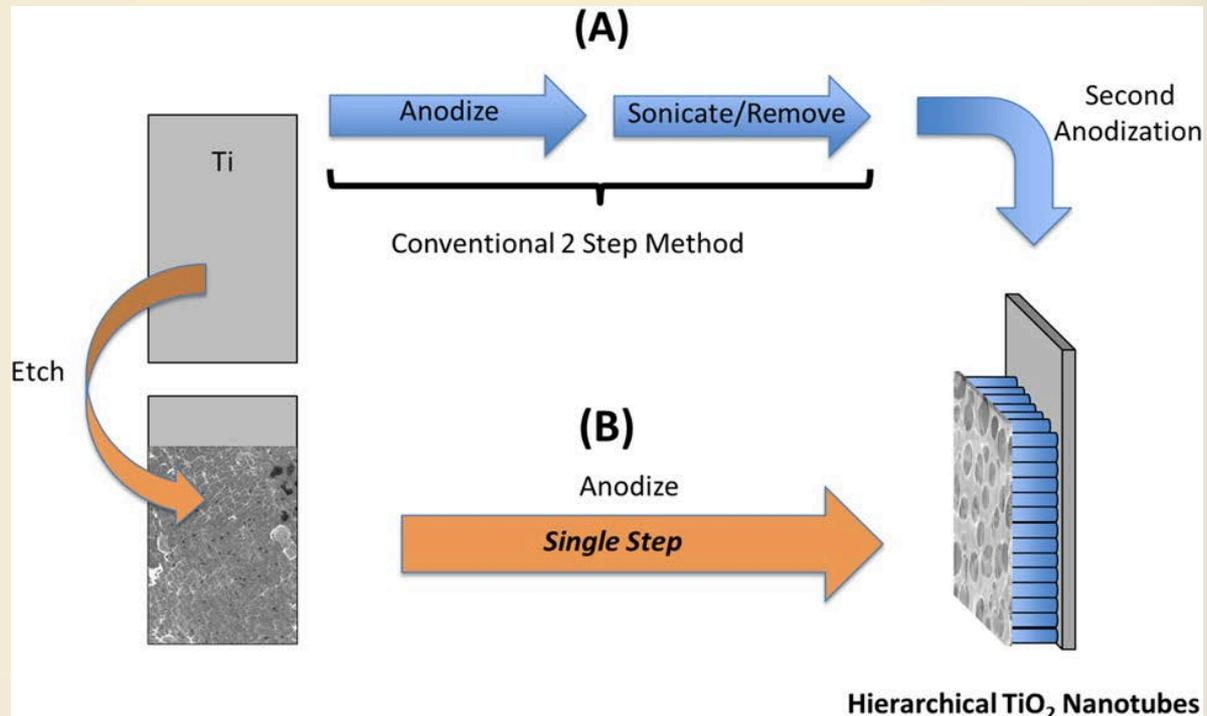
The same top-layered type nanostructure can be obtained by a single anodization process (B) utilizing a surface etching treatment prior to anodization
