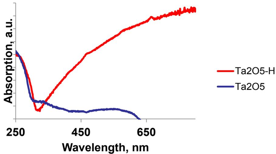
Ta<sub>2</sub>O<sub>5</sub>: annealed in air at 500 °C 2h
