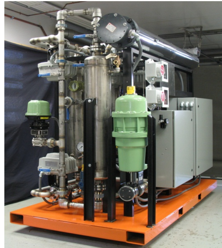
TDA's Biogas Cleanup Skid
