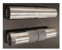
Example of a notched tubular test article that could be used to characterize polymers exposed to high-pressure hydrogen at extreme temperatures, from the laboratory of Wei Yang Lu.
