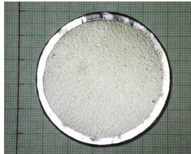
Liner with dimpled or patterned inner surface
