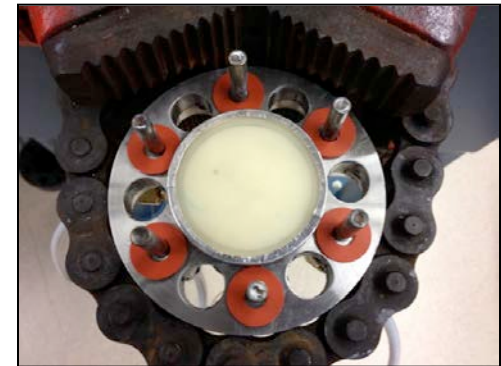
Downstream flange with polymer specimen and metal foil seal folded over edge
