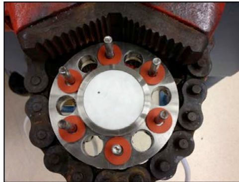
Downstream flange with cartridge heaters and quartz support frit installed
