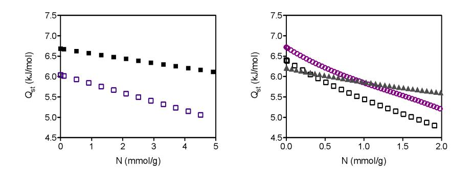
No significant increase in the Q<sub>st</sub> values were observed for Zn<sup>2+</sup> and Mg<sup>2+</sup> metallated materials
