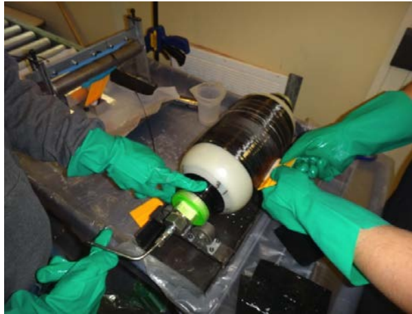
Distribute epoxy resin
