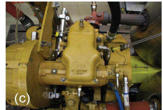
Top: A cut through the cylinder showing the spatial distribution of temperature for different treatments of tunneling; Bottom: Caterpillar single-cylinder test engine
