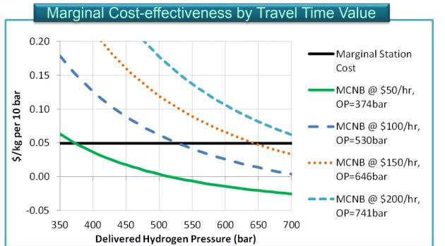
assume: cluster strategy in Santa Monica, 1 stations at 150 kg/day capacity each (3.7% of gas stations), 150 FCVs driven at 1.3k mile/yr, onboard storage cost \$19/kWh at 700bar and \$16/kWh at 350bar. Refueling travel time value varies from \$50/hour to \$200/hour, which is further multiplied by a refueling annoyance factor of 3.5.
