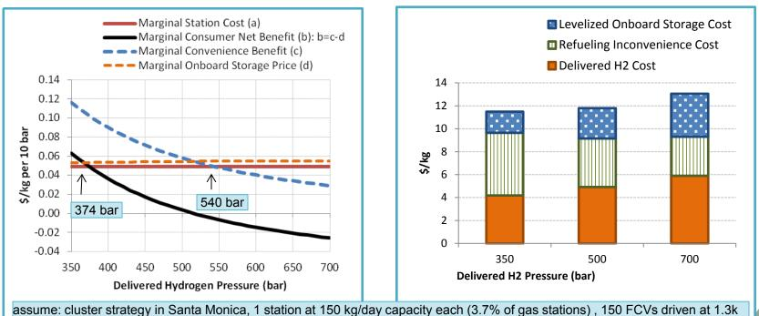
mile/y each, \$50/hr time value, onboard storage cost \$19/kWh at 700bar and \$16/kWh at 350bar
