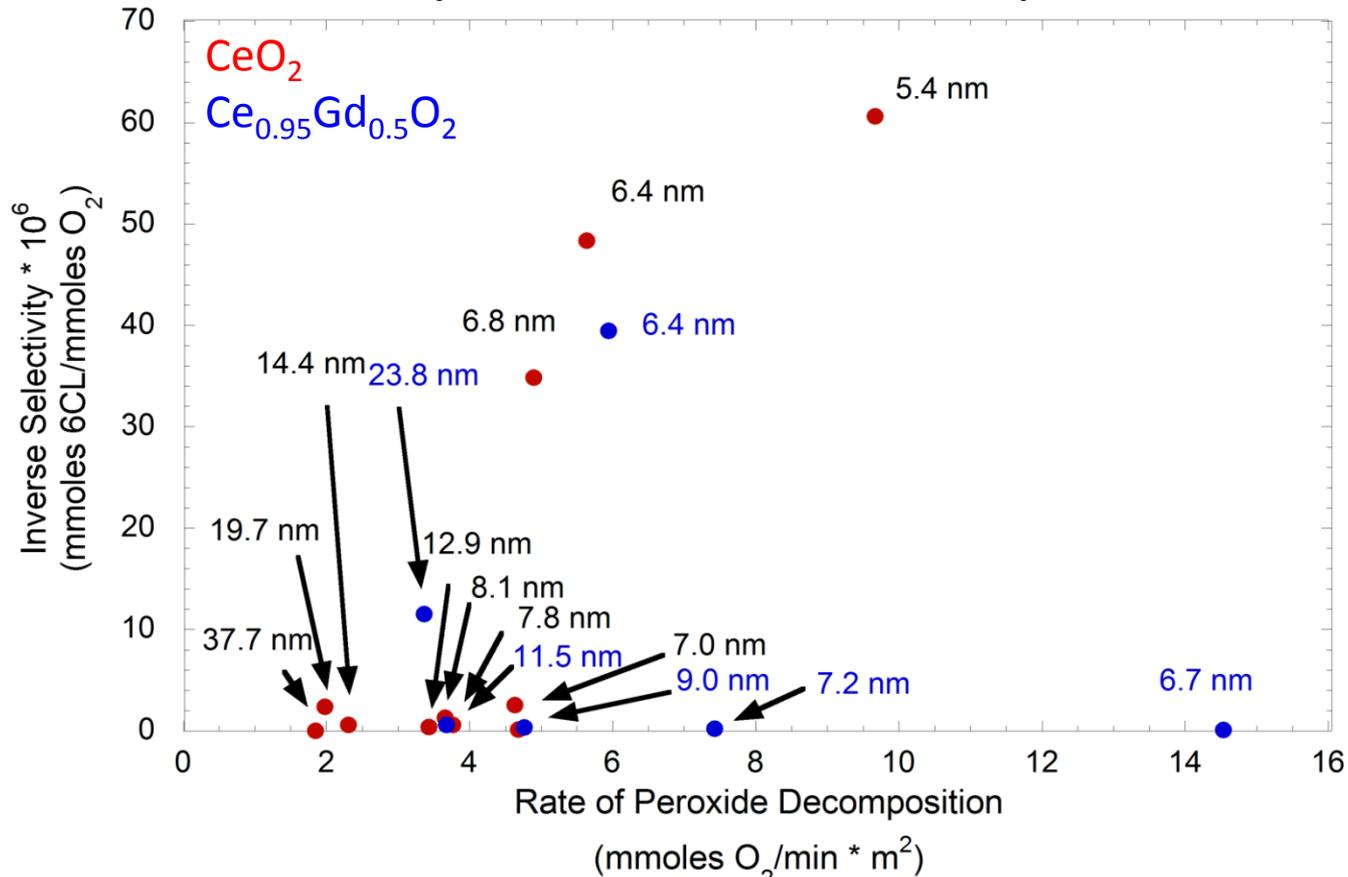
5 % Gd doping of ceria results in high peroxide decomposition rates with lower free radical generation for most particle sizes
