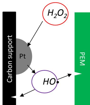
Peroxide generation and degradation into free radicals that attack the carbon support and PEM
