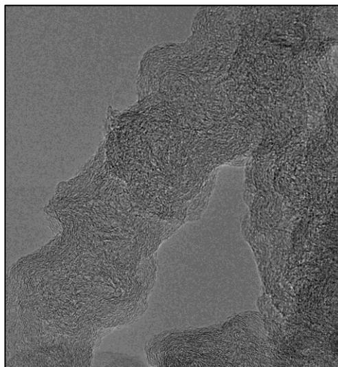
**Pyrolysis:**  $1000^\circ\text{C}$ , 1h
