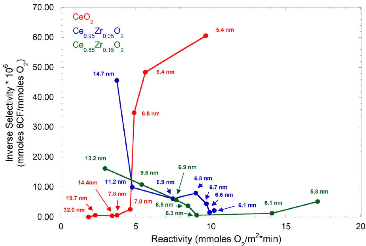
15 % Zr doping of ceria results in high peroxide decomposition rates with low free radical generation for small particle sizes; Zr doping also improves nanoparticle acid stability
