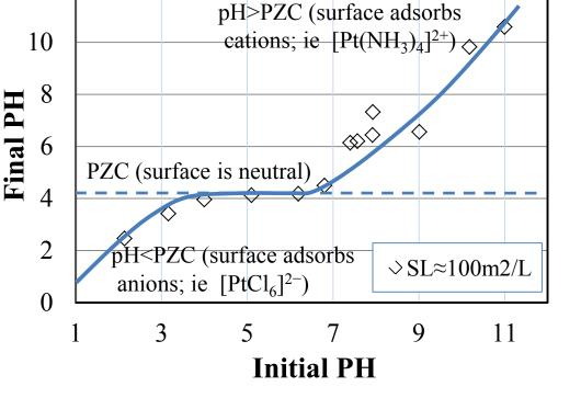
"Strong electrostatic adsorption" (SEA) method was used.
