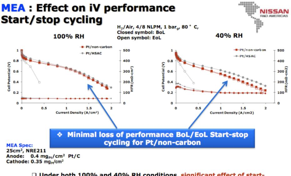
Under both 100% and 40% RH conditions, significant effect of startstop cycling observed for Pt/HSAC
