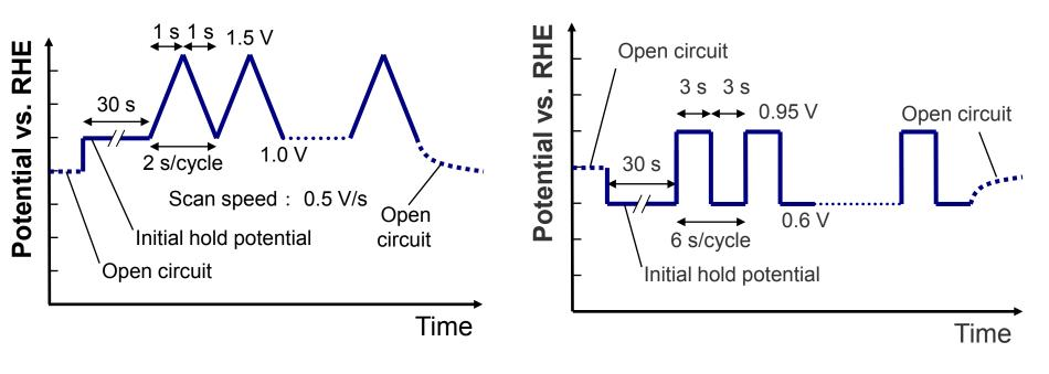
Support Durability—Support corrosion
