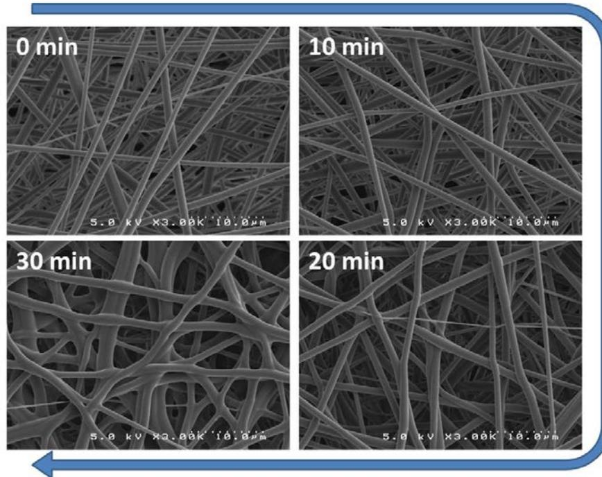
Interfiber welds start to form between 20-30 minutes of room temperature exposure of the mats to DMAc vapors.
