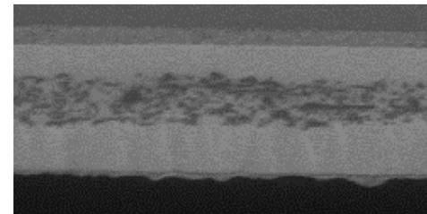
Ionomer/Fiber composite center layer with ionomer skin layer
