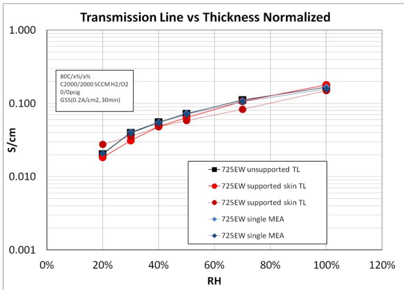
Membrane Conductivity from HFR data (Z-Axis)
