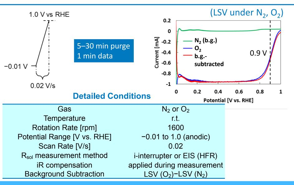
0.90 V vs. RHE, 25°C, 100 kPa, 1600 rpm, O<sub>2</sub> saturated 0.1 M HClO<sub>4</sub>.
