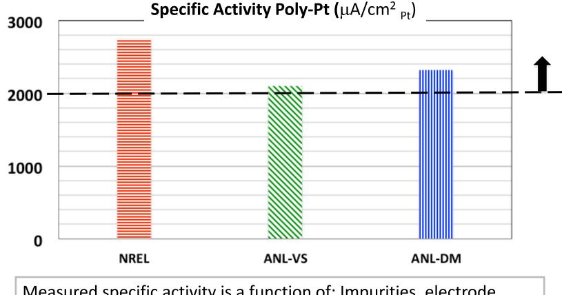
Measured specific activity is a function of: Impurities, electrode surface preparation and electrochemical conditioning.
