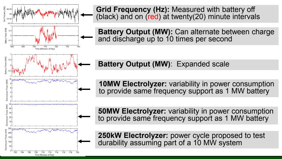
Frequency variability on 150MW grid system reduced with a 1MW, 250kwh fast BESS. Same power range as 1MW BESS easily achieved with 'low' stress and good CAPEX utilization using MW-scale electrolyzers.
