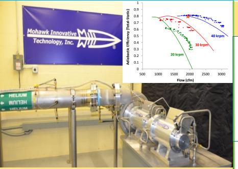
Verified the potential of improved centrifugal pipeline compression to reduce compression capital cost to \$2M from \$2.7M in 2013. Based on a 3,000 kW motor rating
