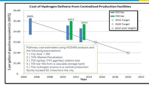
Range of HDSAM projected costs of hydrogen delivery from central production facilities in 2005, 2011, and 2013 along with the relevant targets.
