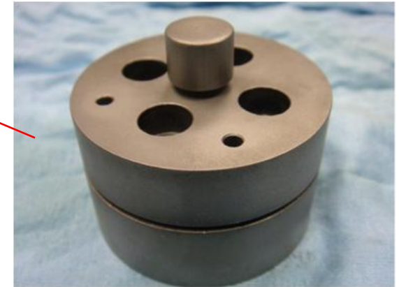
Specially machined fixture for small hole punch testing of metal specimens for project tests at speeds of 0.0021 mm/s
