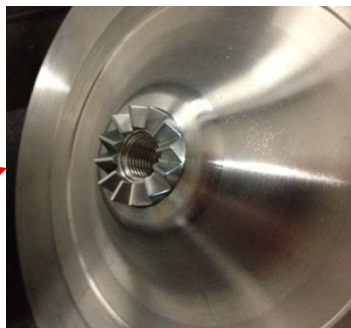
Curvic Spline Couples Rotor to Drive Shaft
