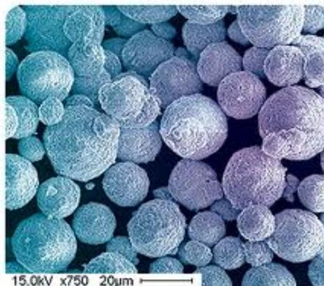
Spray dried particles can operate up to a calculated lifetime of 396,000 cycles based on 1000 °C; 1000 hr runs for chemical looping combustion: (= 3.75 yr lifetime for \$2/kg H<sub>2</sub> target)
