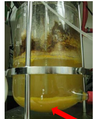
Settled lignocellulose retained acclimated microbes
