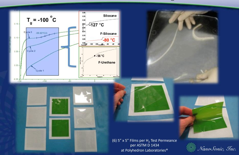
NanoSonic Triple Cold Flex Test for H<sub>2</sub> Permeance Specimens at -50 °C on Hose Materials: Shown Flat, Mid-Way, and at 180 ° Fold
