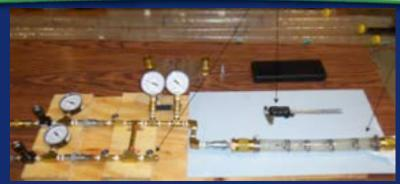
Hydrostatic Strength (section 2.4) of ANSI/CSA HGV 4.2-2013
