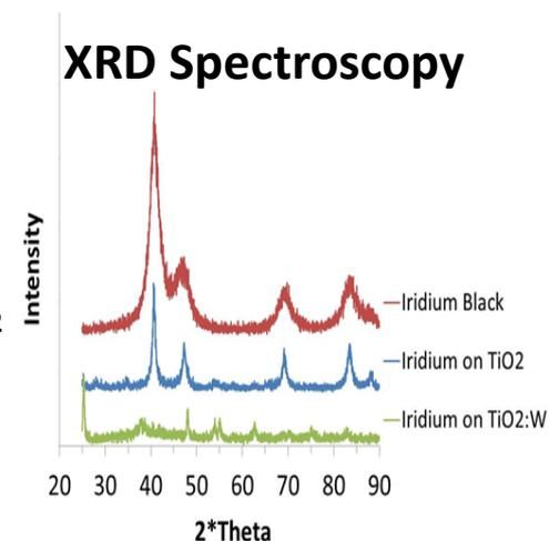
Nano-sized Ir on various supports have been synthesized via chemical deposition
