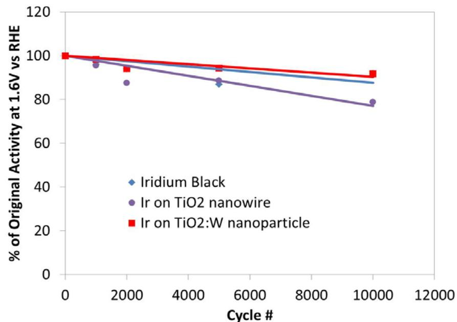
**Scan rate:** 50 mV/s; **RPM:** 1960 rpm; **Ir loading:** 40-80  $\mu\text{g}/\text{cm}^2$ ; **Solution:** 0.5M H<sub>2</sub>SO<sub>4</sub>
