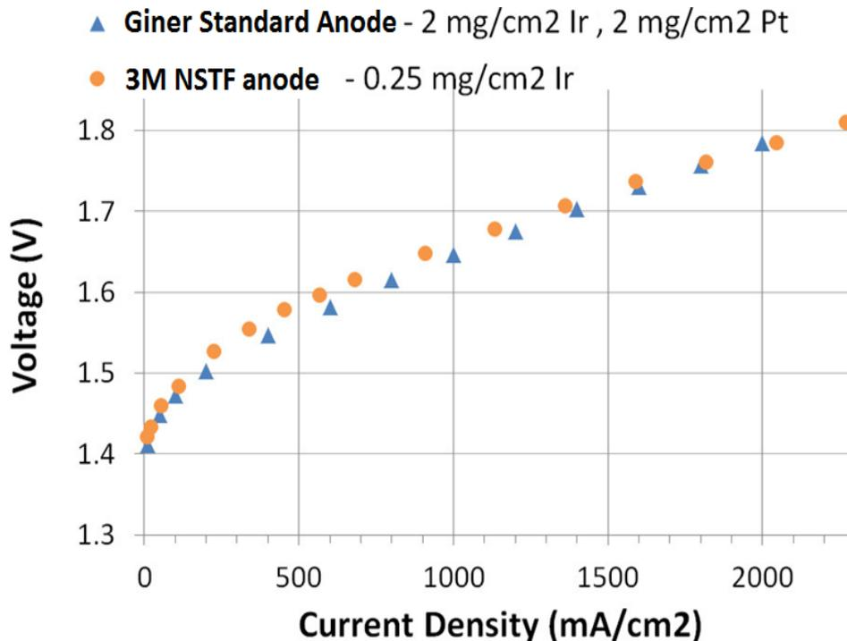
3M IrNSTF anode demonstrates comparable performance to standard anode but at 1/8 Ir loading and 1/16 PGM loading
