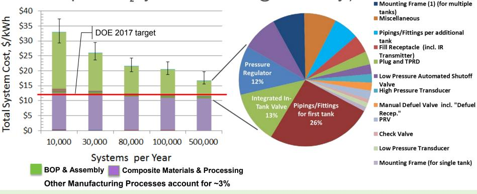
Piping/fittings, integrated in-tank valve and pressure regulator are the high cost items for BOP (SA – ST100)
