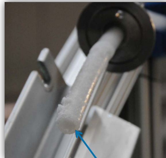
Viscous AB filled the 1/2 in Teflon tubing
