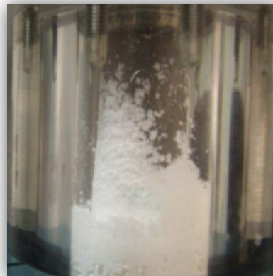
Filter caking after 20 slpm N 2 fluidized MOF-5
