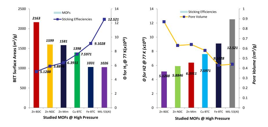
The graphs show that there is an inverse correlation between Surface Area/Pore Volume and Sticking Efficiency ( $\theta$ ) of H<sub>2</sub> on the various MOFs. A similar correlation exists for the adsorptions of CH<sub>4</sub> and CO<sub>2</sub>.
