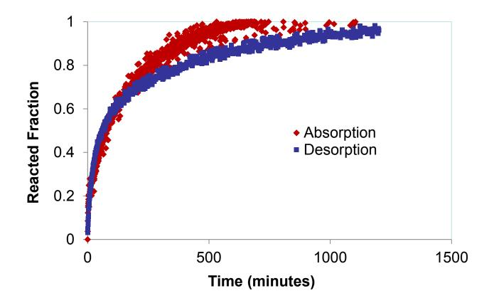
Kinetics were done in the two-phase region at 160 °C and N=3. The results show that absorption occurs faster than desorption under the same conditions. It takes ~350 minutes to attain 90% absorption whereas ~740 minutes are required for 90% desorption.
