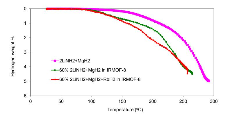
The TPD plots show that nanoconfinement of  $LiNH_2/MgH_2$  in IRMOF-8 causes hydrogen to be released at a lower temperature. Doping with  $RbH_2$  produces a further lowering of the desorption temperature.
