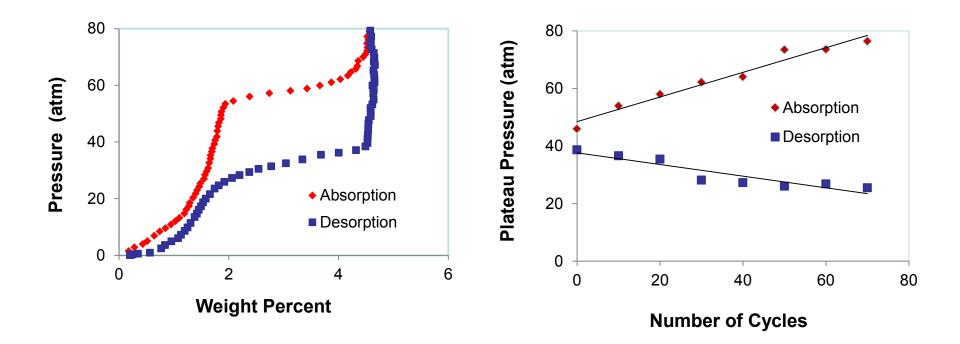
The absorption and desorption PCIs shown above on the left were done at 160 °C after 20 cycles. The plots show that there is a significant amount of hysteresis. The graph on the right gives the absorption and desorption plateau pressures after every 10 cycles up to 70 cycles. It is evident that the hysteresis increases as a result of cycling.
