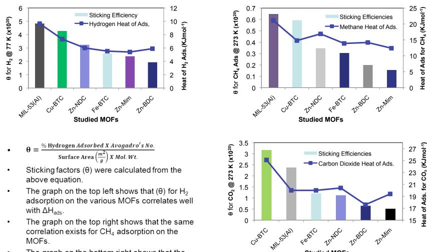
The graph on the bottom right shows that the ٠ same correlation exists for CO<sub>2</sub> adsorption on the MOFs.
