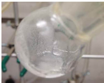
fuel blend BEFORE desorption (single phase at <80 °C)
