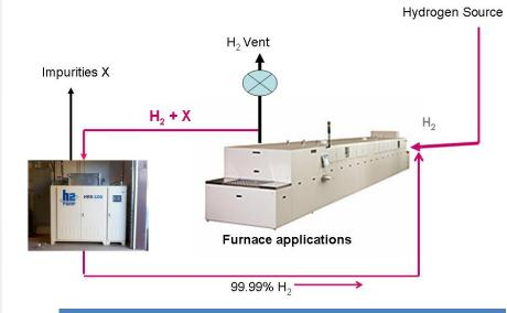
Industrial operations flare or vent hydrogen rich furnace exhaust gas into the atmosphere today The HRS-100 can cost effectively reclaim, purify and pressurize the hydrogen exhaust
